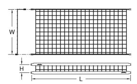
**Weight Capacity** Our Wiremesh Shelves have passed static load tests of up to 200 pounds per shelf (tested using equally-distributed loads upon the shelf). Additional weight can be accommodated by using rebars for support.
