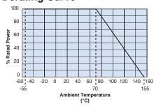
For resistors operated at an ambient temperature of 70°C or above, a power rating shall be derated in accordance with the derating curve.
