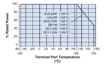
For resistors operated at an ambient temperature of 70°C or above, a power rating shall be derated in accordance with the derating curve.
