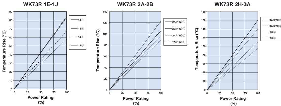
Regarding the temperature rise, the value of the temperature varies per conditions and board for use since the temperature is measured under our measuring conditions.
