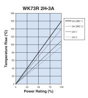
Measurement condition Room temperature: 25°C PCB: FR-4t = 1.6mm Cu foil thickness: 35μm
