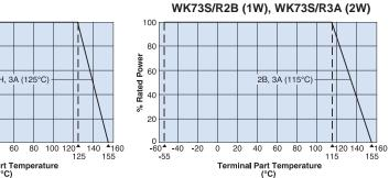
For resistors operated terminal temperature of described for each size or above, a power rating shall be derated in accordance with the derating curve.
