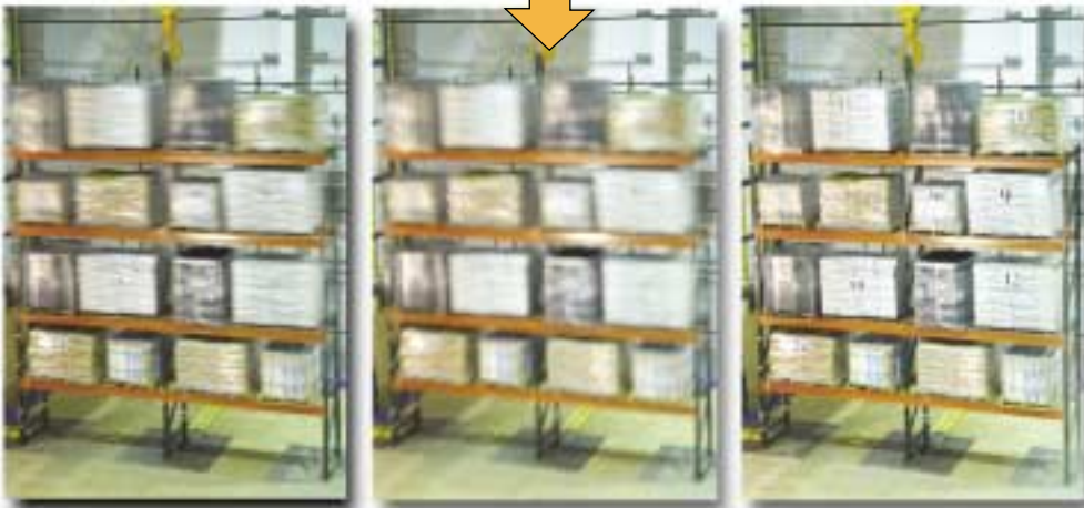
RIDG-U-RAK's Base Isolated System during the same 30 second AC156 200% Earthquake Simulation
