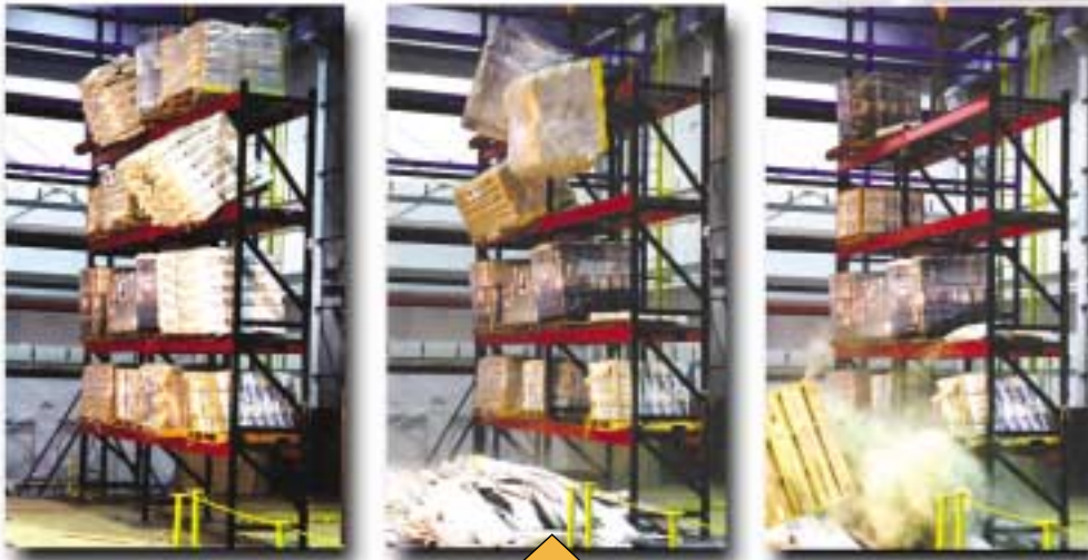
Conventional Fixed Rack during a 30 second AC156 200% Earthquake Simulation
